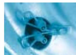
Flexible extensions and holder used on dual wheels
